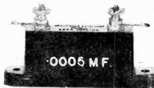
Trix fixed condenser with terminals and soldering tags.
